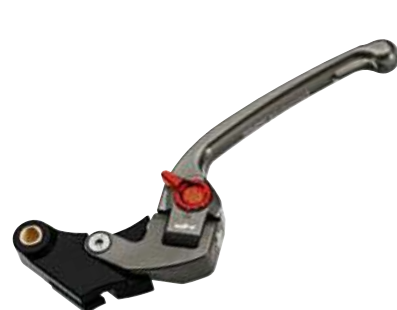
2 Folding HP clutch lever
