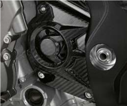
5 HP carbon sprocket cover
